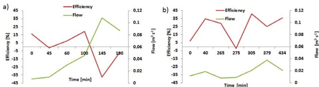
Fig. 6. The impact of flow volume on SSBS purification efficiency; a) storm event on 30.03.2012; b) storm event on 31.03.2012.
