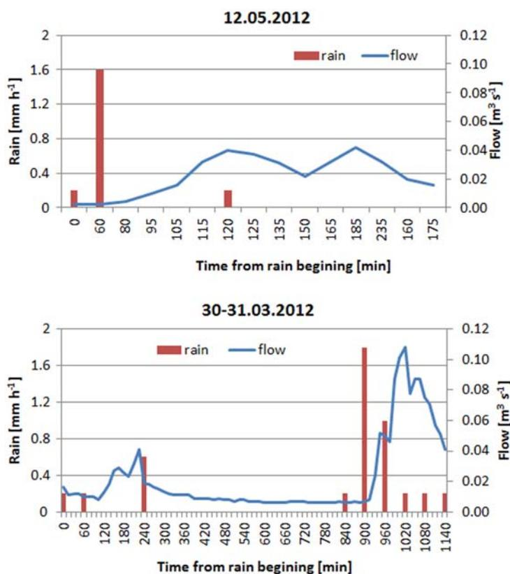
Fig. 4. Rain and flow comparison on SSBS for three analyzed storm events.
