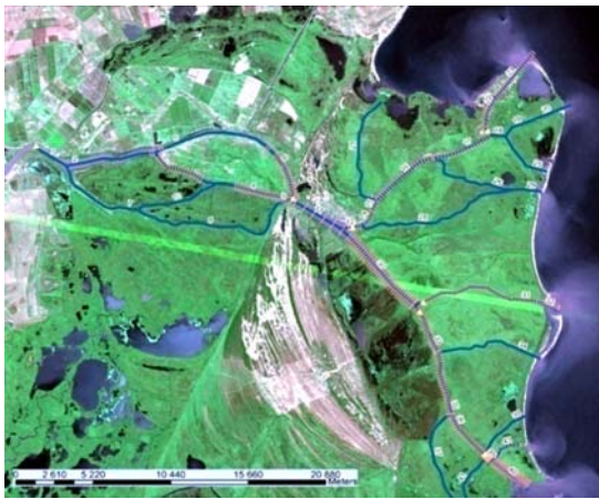
Fig. 3. The part of Romanian and Ukrainian Danube River Delta near Vylkove and C.A. Rosetti modelled within the USRIEP project. Arrows indicates Bâstroe, Chilia, and Starostambulske branches of the delta river network with computational sections and hydrological stations.
