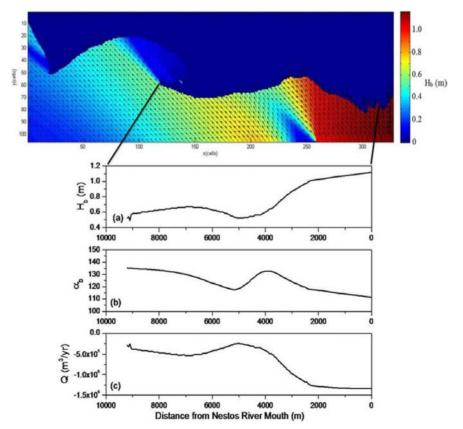
**Fig. 10.** SWAN model results showing incident wave heights and angles (upper panel) and longshore distribution of (a) breaking wave height (m), (b) breaking wave angle (o) measured from the x-positive (east) axis in an anticlockwise manner, and (c) longshore sediment transport ( $m^3 yr^1$ ) at Keramoti shoreline (lower panel).
