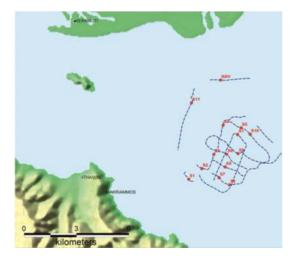
Fig. 3. Sea bottom coverage using bathymetric and side scan sonar systems. Points represent van Veen surface sediment samples.
