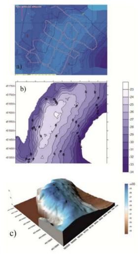
**Fig. 6.** a) Contours of sea bottom bathymetry and survey lines in the area of interest, b) Contours of sea bottom bathymetry produced using ArcGIS, and c) three-dimensional view of the sandbank.
