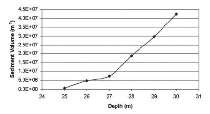
Fig. 8. Estimation of sediment volume excavated from seabed for beach nourishment.
