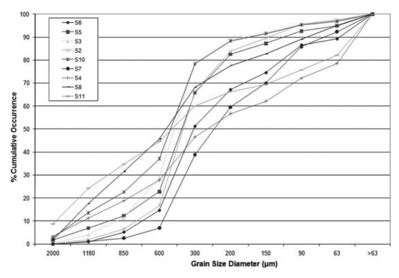
Fig. 7. Curves of cumulative occurrence of grain size distribution for all bottom samples.
